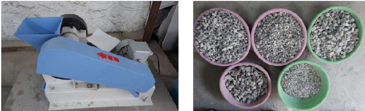
Fig. 3-4. 10 & 20 mm aggregate preparation at Lab scale.
